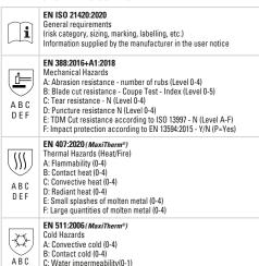
Higher values stand for better protection/resistance. If "X" is marked as a performance level the test is either not applicable or not proceeded. Puncture resistance should not be confused with piercing exerted by thin tips or needles.
